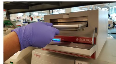
Figure 47: Placing chamber in oven
