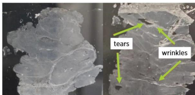
FIGURE 4: GOOD (LEFT) AND BAD (RIGHT) SECTIONS MOUNTED ON A SLIDE
